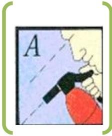
**AIM:** The nozzle horn at the base of the flame.
